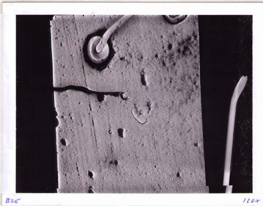
SUBSTRATE WIPED ACROSS WITH FINGER TO INTRODUCE ORGANIC CONTAMINATION
